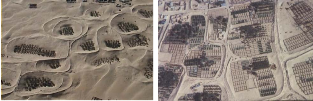
fig: the system of Ghotts Irrigated agriculture without pump and hoses = an ingenious system (A know how / Fight against silting) 2
